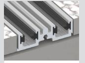
Flush sill with disability access compliance, running track is protected from damage.
